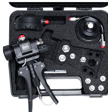
P/N PV411-104-HP-1-XXX hand pump kit with DPI 104 digital test gauge (gauge pressure range to be selected when ordering).
